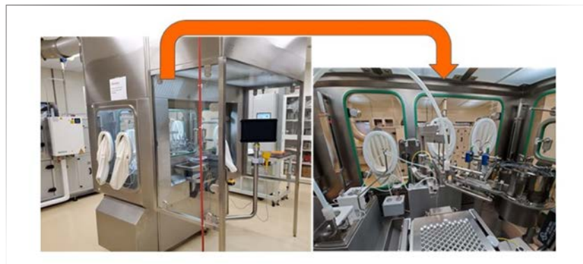
Figure 1. Visual of a custom-designed small-scale syringe and vial filling and stoppering system.
