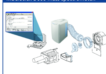
Figure 3: Selectra installation on the MDS/Sciex 3000 mass spectrometer.
