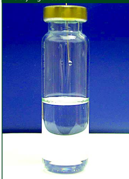
Figure 1: A 1 µL droplet of extracting solvent on the tip of a #2 bevelled microsyringe needle.
