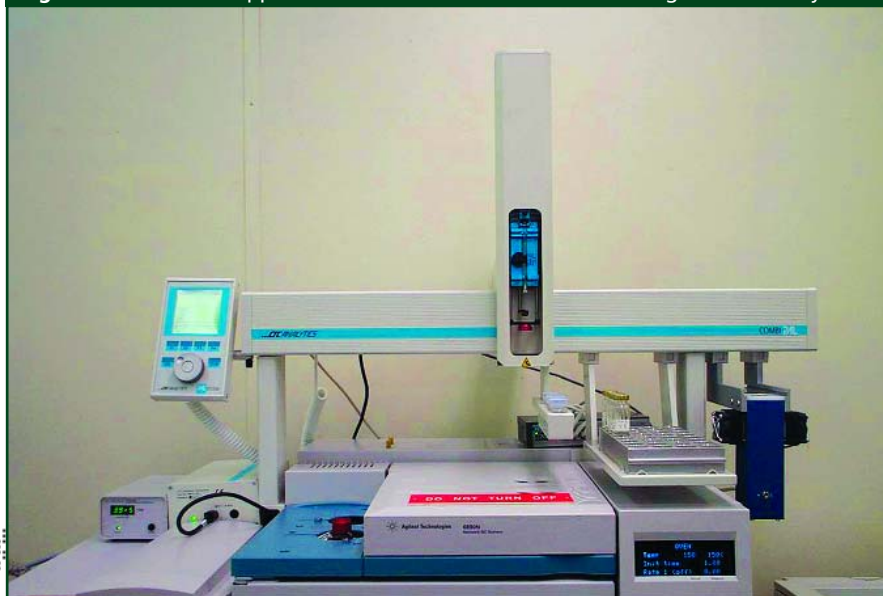
Figure 2: Automated apparatus: CTC Combi PAL installed on an Agilent GC-MS system.
