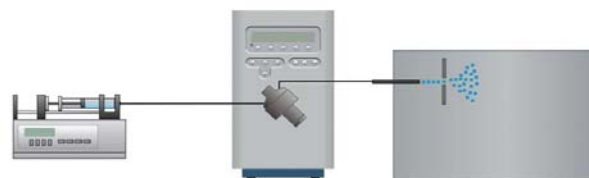
Fig. 2. ROXY™ EC System including ReactorCell™ and dual syringe infusion pump.
