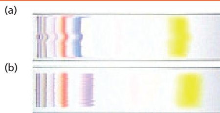
Figure 6: Close-up of dye molecules at column wall during a chromatographic separation with (a) non-FEW and (b) FEW instruments.
