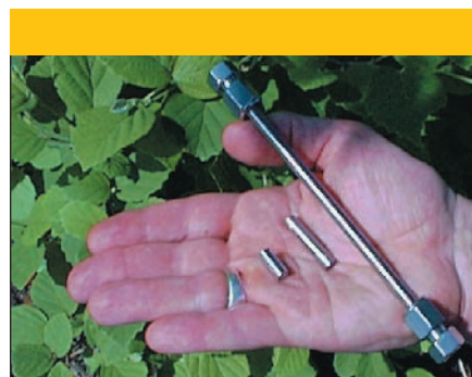
Figure 5: Photograph of a regular-length HPLC column (25 cm) and short, fast 1- and 3-cm HPLC columns. (Courtesy of Agilent Technologies.)
