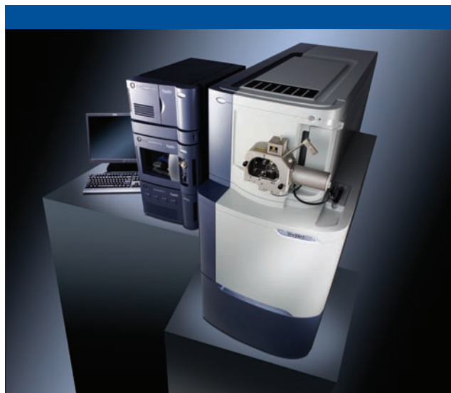
Figure 1: The Waters ACQUITY UPLC system with the Synapt High Definition Mass Spectrometry system.
