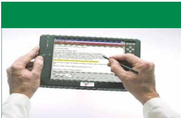
Figure 1: A digital version of a standard operating procedure (or method) is presented to the QC lab analyst or production floor operators with automatic capture of critical method-based data. This process eliminates transcription errors associated with paper-based notebooks.
