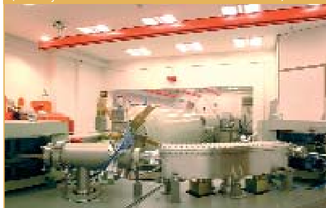
Figure 1: The accelerator mass spectrometer at Oxford (courtesy of the Oxford Radiocarbon Accelerator Unit).
