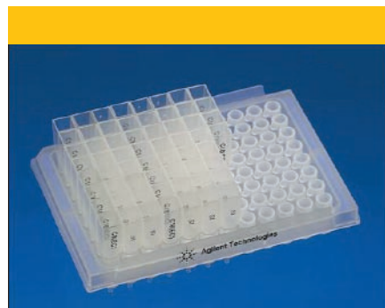
Figure 4: Photograph of a flexible 96-well SPE plate with removable cartridges and plug strips. (Courtesy of Agilent Technologies.)
