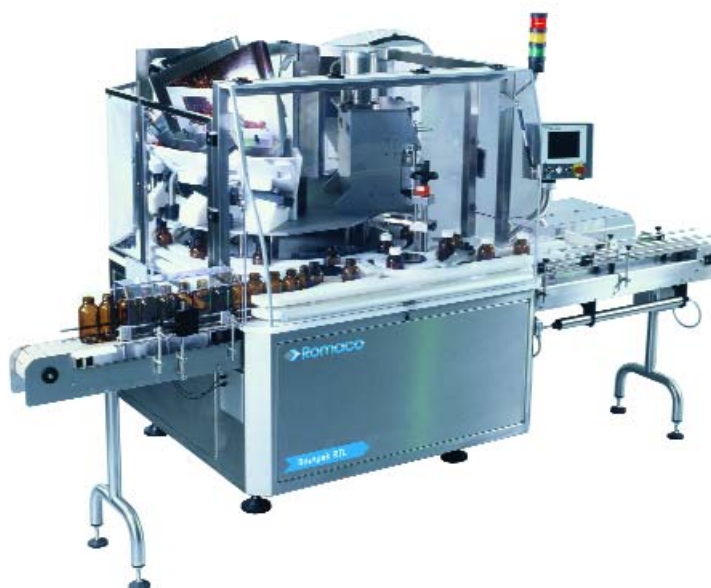
Figure 1 The compact monobloc from Romaco counts tablets and caps containers at a rate of up to sixty 100-count bottles/min.
