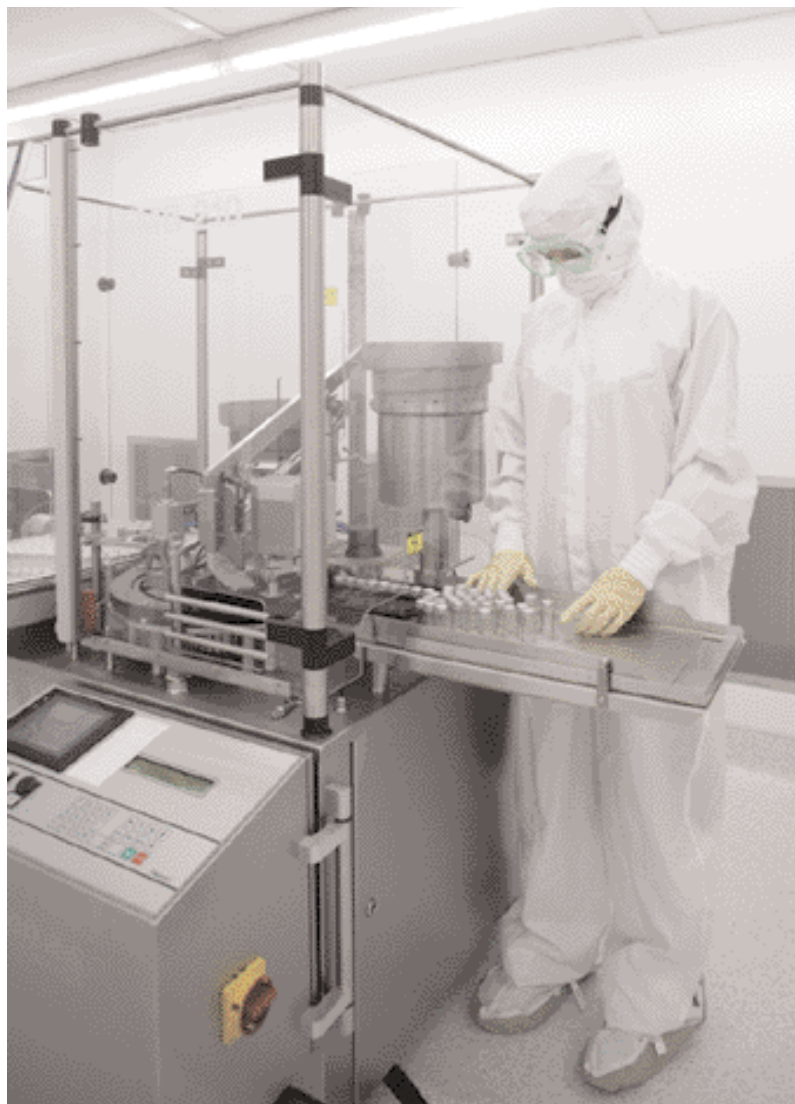
An Althea Technologies laboratory technician with the Flexicon Monoblock automated vial filling machine.
