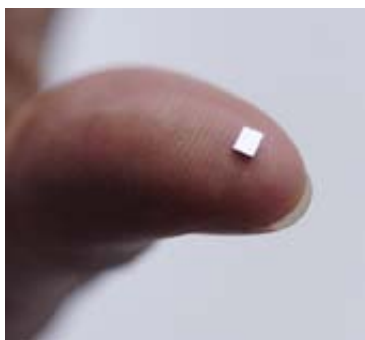
Figure 1: Cypak's microelectronic sensor chip is about 0.3 mm in height and can store 32 kilobytes of memory.
