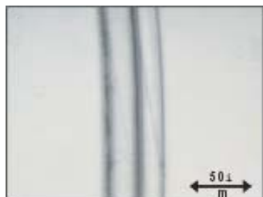
Figure 2. Bright field image of the multi layer sample. Cross section of 4 layer laminate film Thickness: 3 \mu\text{m} (Picture taken with internal CCD of UMA600)
