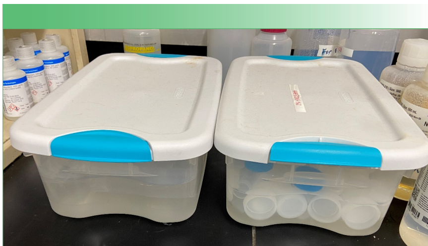
FIGURE 2: ICP-MS sample introduction components are cleaned and stored in separate containers for different kits (for example, standard quartz and PFA inert kit components).
