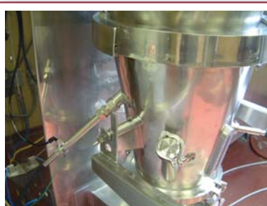
Figure 1. The 1-in. NIR probe is inserted in the port at a 45° angle in the product container of the fluid bed dryer.
