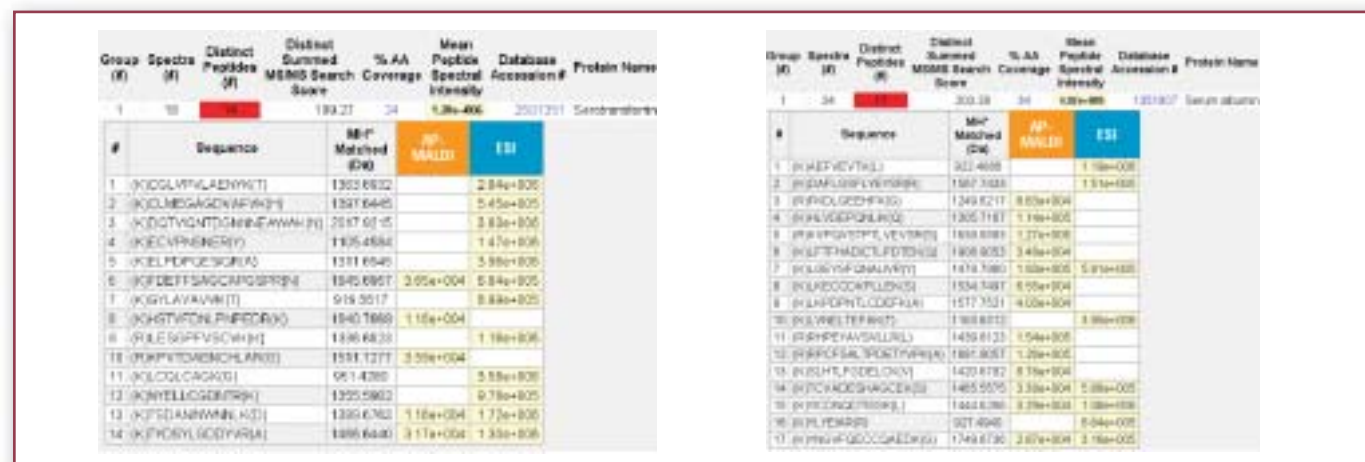
Figure 6. Comparison of AP-MALDI and ESI data files. Combining data from both techniques improves sequence coverage in protein digest analysis because each type of ionization produces some unique peptide identifications. In the examples shown here, ESI provides superior sequence coverage in the analysis of apotransferrin than AP-MALDI, while the reverse is true, but somewhat less dramatic, for BSA. (Image courtesy of Agilent Technologies, Palo Alto, CA.)
