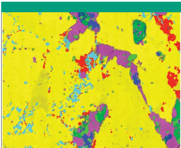
Figure 3: Granite - Al-cyan; Si-yellow; K-red; Ca-green; Mn-blue; Fe-magenta.
