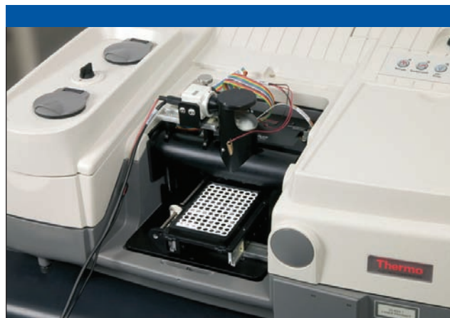
Figure 1: Micro Well Plate Reader installed in a Nicolet 6700 FT-IR Spectrometer.
