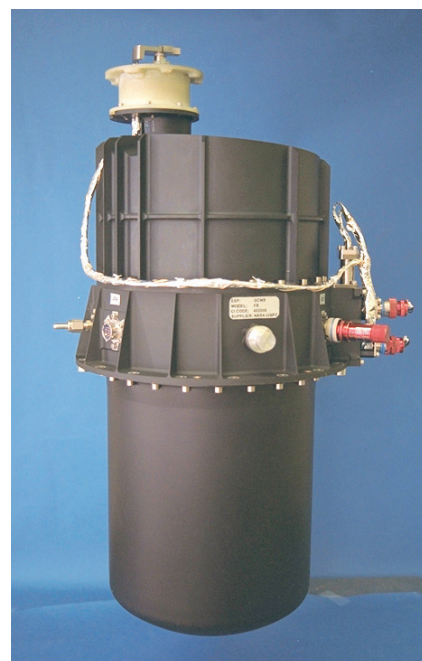
The upper half of the GC-MS system seen in this picture includes the sampling system and the ion sources, and the lower half covers the electronics system. The gas inlet port is at the very top, at the dome of the housing.
