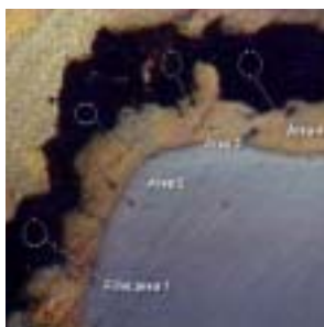
Figure 1. Crack section as viewed through the Raman microscope (500x).
