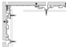
With the side clip, the width of the slat can be narrowed by up to a half. In this case the slat must be re-drilled
