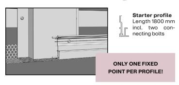
First fixing of the profile with drilling screw (fixed point). For further attachment points (floating points), the profile must be pre-drilled (diam. 4.5 mm). For a profile joint (min. 3 mm), the thermal expansion is ensured via the connecting bolts. The starter profile must be mounted horizontally and start at the same height everywhere.
