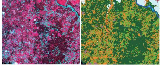
a b SPOT RGB (3, 2, and 1) image (a) and its corresponding land cover Classification (b).
