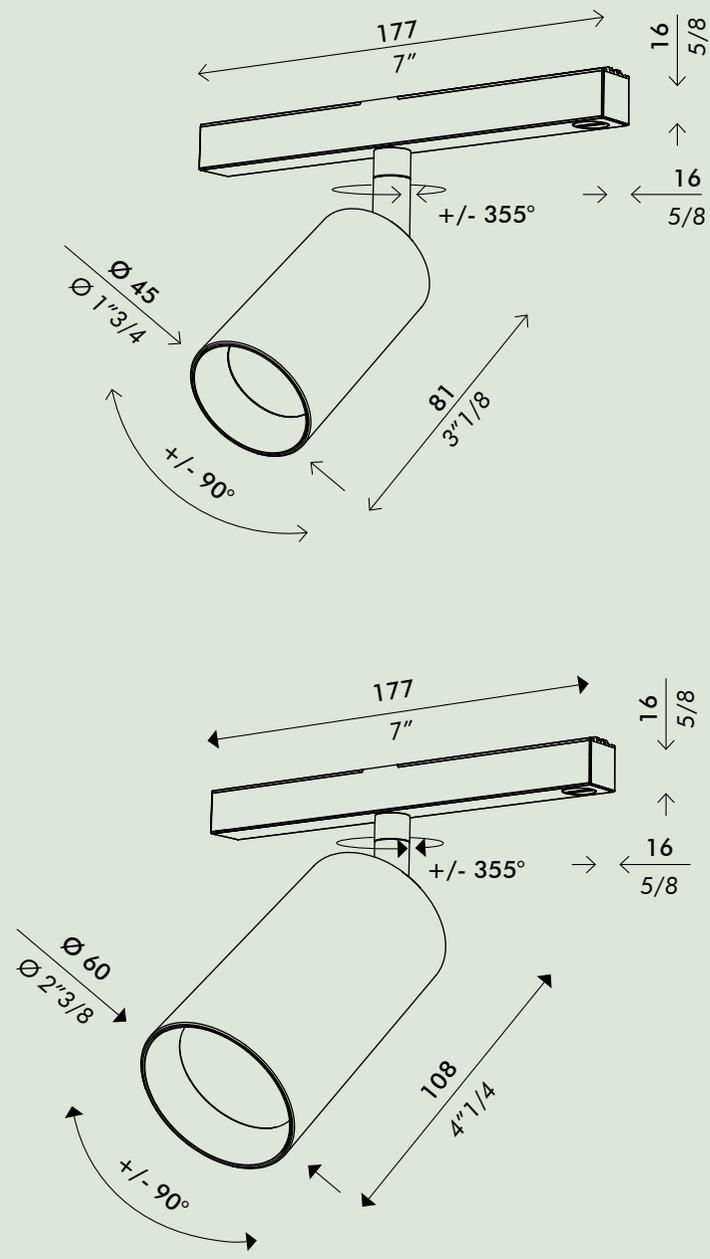
cyl track 48V Ø 45cyl track 48V Ø 60
