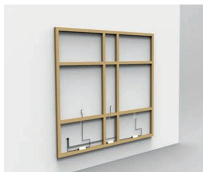
1. Create the supporting frame and provide for power connections for the individual letters.
