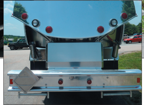
Rear view of partial rear canopy with meter box.
