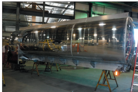
Finishing - this is the final stage of tank production process where all components are assembled on the vessels.
