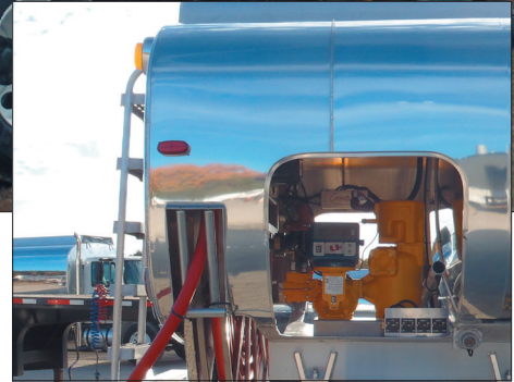
Metering equipment on platform installed between tank long sills.
