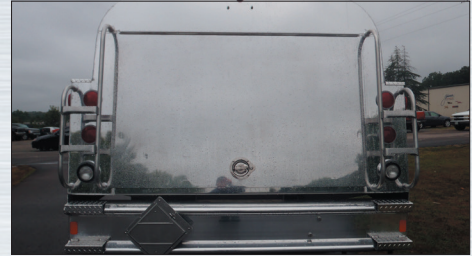
Combo Style tank ladders that go halfway up the tank side to access the side catwalks.
