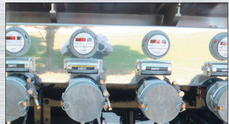
Electronic liquid level indicator with small screen readouts that can be installed on the outside of the tank or inside the cab of the chassis.
