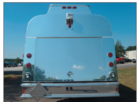
Rear enclosed bucket box with uplifting door.
