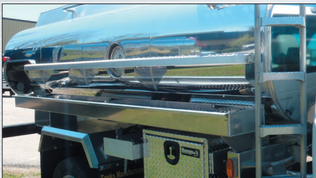
6" wide side catwalk made of grip strut with grate style openings.
