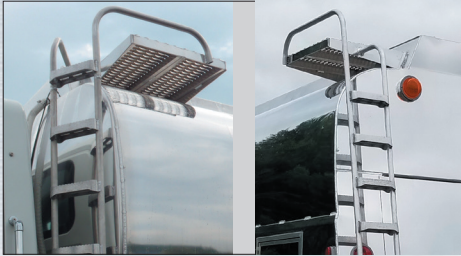
Standard ladder can be used on any corner of the tank with a small casted step and top grip strut platform.
