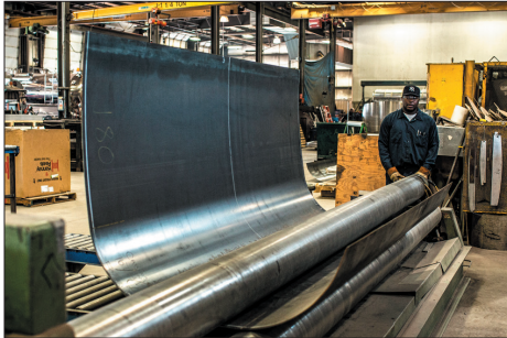
Fabrication - this process starts by taking a flat sheet of metal, then it is rolled to create the side shell tank shape.
