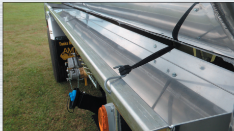
Standard side hose trough made to specific width and length
