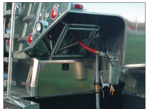
Rear frame mounted meter box installed under rear canopy to house meter and compartment switches.
