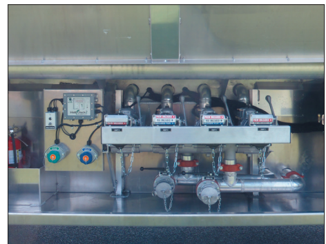
Side cabinet that houses all tank piping.
