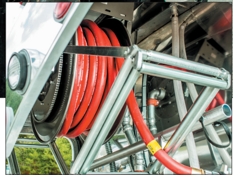
Hose reel inverted under canopy – four way roller rack system
