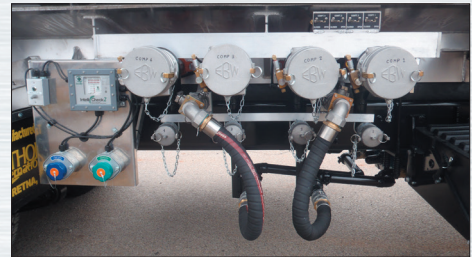
Piping option with compartment lines to the curbside for bottom loading and "T" down for dry brakes.
