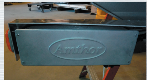
Large watertight casted aluminum electrical box installed on front driver side of the tank.
