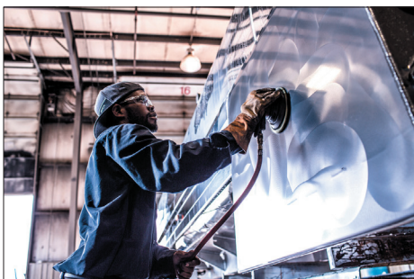
Cleaning - Final stage of the manufacturing process. Blemishes and imperfections are cleaned and polished at this point.
