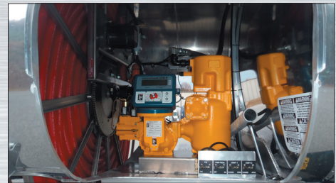
Single wrap hose reel system.
