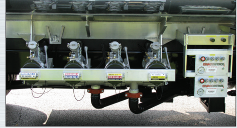
Piping option with compartment lines to the curbside air operated manifold with product returns and full bottom loading.
