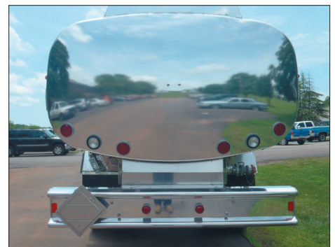
Rear view of the full rear canopy with meter box.
