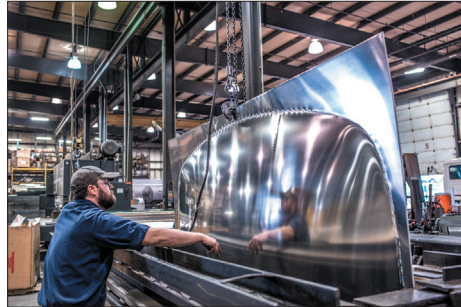
Heads - the heads and baffles of your tank are either air blown or formed with a shear and break to the specific size of your tank.
