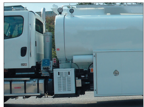
Stainless Steel DEF Tank mounted along side an aluminum tank.
