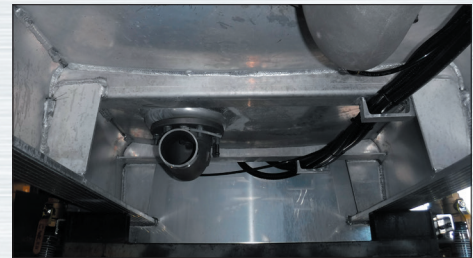
Both sides of the longmembers are tied in to the horizontal floor brace to strengthen the tank.
