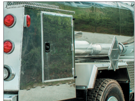
Side access doors to rear bucket box (available on both sides of the tank).
