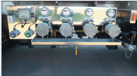
Piping option with compartment lines to the curbside for bottom loading only. Additional lines to the rear for dry brakes are available.
