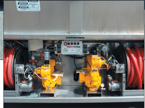
Cabinet that houses metering and hose reel equipment.
