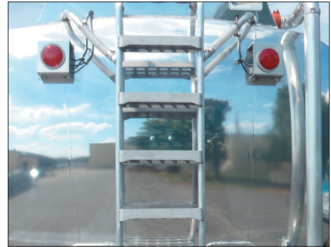
Rear ladder with built in drains from top overturn.
