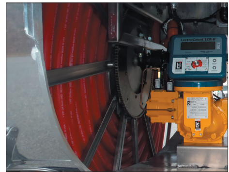
Inverted single wrap reel or multi wrap hose reel with a four way roller rack system
