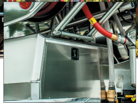
Metering equipment installed in a meter box between the frame rails of truck chassis.
