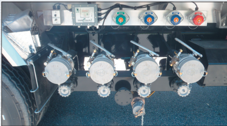
Piping option with compartment lines to the curbside Amthor exclusive manual valve operated manifold with full bottom loading.
