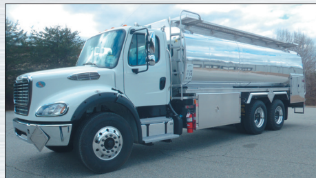
Top catwalk available in 12" or 18" wide made of grip strut with grate style openings.
