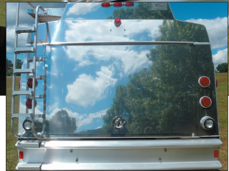
Rear enclosed bucket box with uplifting door.
