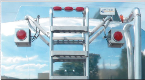
Rear ladder with large casted steps and built in drains from top overturn protection.
