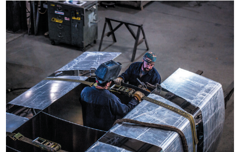
Fixture - this is where the tank assembly begins. The side shell, top, floor, and interior of the tank are assembled and tacked together on a fixture model of a truck chassis.
