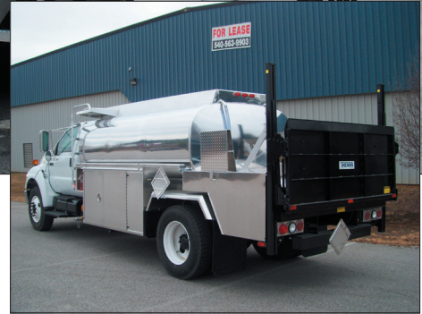
Specialized equipment refueler with liftgate and platform to carry spare tires.
