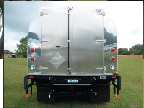
Rear view enclosed lube liner with barn style doors.
