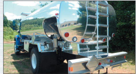
Standard rear ladder with large casted steps and no rear drains.
