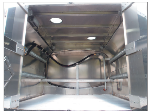
Inside view of aluminum extruded floor and E-track.
