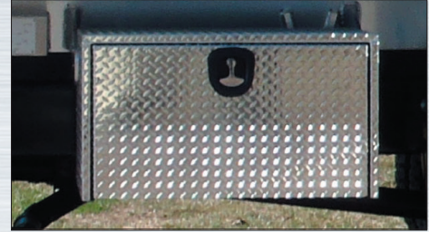
Standard toolbox with single drop down door.
