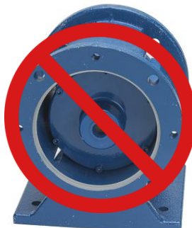
2. Always ship the outer magnet separately from the pump assembly. Shipping as shown above will cause damage to the magnets.
