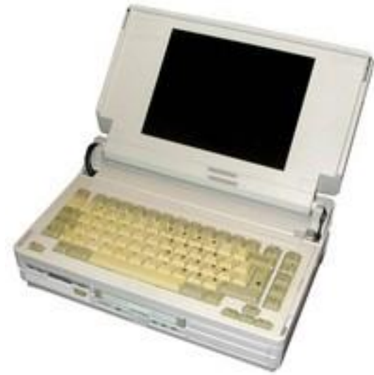
The Compaq SLT/286, 1990 VGA, 12MHz processor, battery Kilde: computerhistory.org.uk
