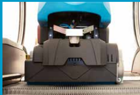
Automatic sensor controls brush deck manoeuvre
