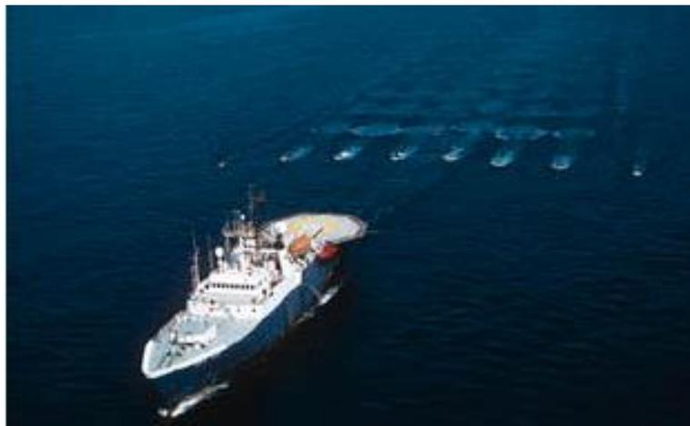
**Figure 2. Photograph of a seismic vessel, the emission sources, the seismic cable (streamers) and the tail buoy.**
