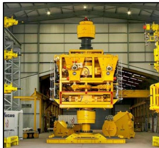
Figure 4: Capping stack
