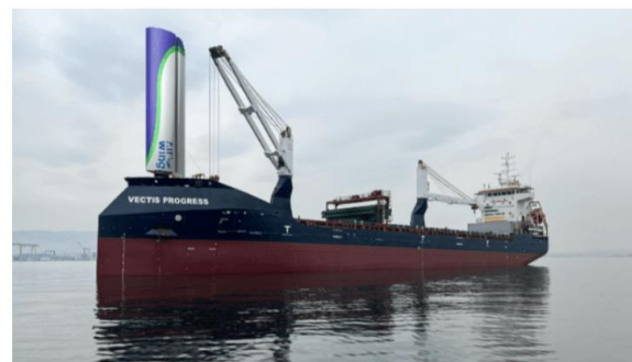
Artist's impression of a 20-metre AirWing™ unit to be installed on Carisbrooke Shipping's general cargo vessel.
