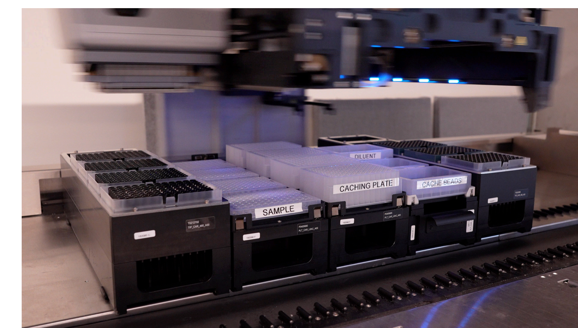
Hamilton Microlab STAR processing 384 samples across four plates
