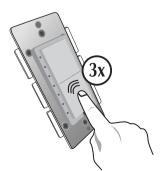
If you see the lighting turns OFF and then ON, it means that the module has been reset successfully and you may retry Step 5 above to add the module into vour network. Otherwise, please repeat the manual reset procedures.
