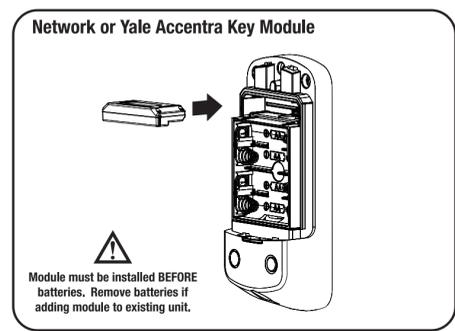
Module must be installed BEFORE batteries. Remove batteries if adding module to existing unit.
