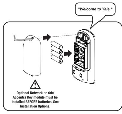
Optional Network or Yale Accentra Key module must be installed BEFORE batteries. See Installation Options.
