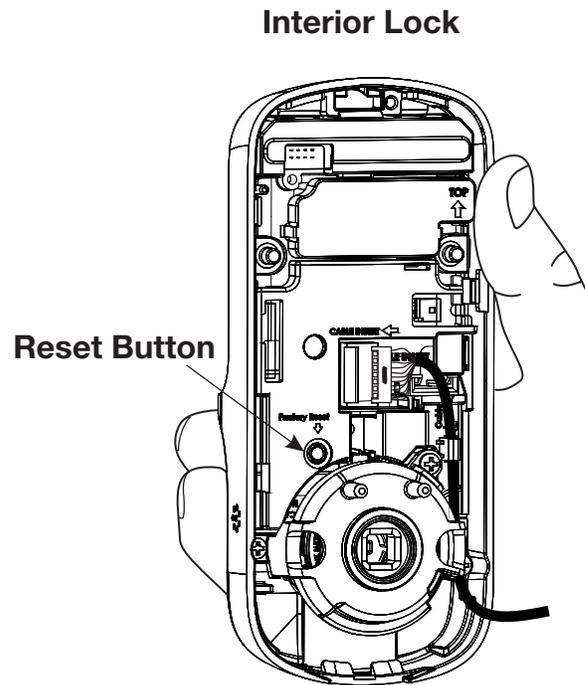
When resetting the lock, all user codes, including the Master Entry Code\*, are deleted. All programming features are reset to original default settings. See “Factory Settings”.
