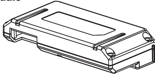
**IMPORTANT:** the batteries must be removed prior to removing and/or inserting the network module:
