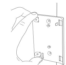
Use the bracket and tape or screws
