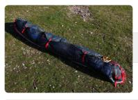
**Step 9.** Turn the Saucisse on its side and make the first fold just after the LE reinforcements. Do not fold the plastic reinforcements, use 3 or 4 folds around the LE.
