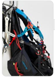
Please note; short bridle parachutes must be attached to the harness bridles (sold separately). If you have a parachute with long Y bridles, these should be attached directly to the shoulder points.
