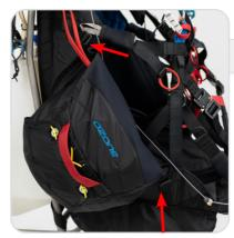
The reserve pocket needs to be zipped into the side of the harness and locked with the plastic buckles to prevent the zips from becoming undone.
