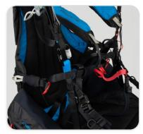
Please see above for connection details with the power unit. If free flying with the Indy, attach the wing's risers to the carabiners at the main hang points. The A risers should be facing to the outside.
