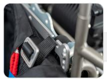
The first method involves using two webbing straps and metal buckles located on the top of the harness. These straps are designed to wrap around the paramotor frame. Always double lock the buckles with the strap.
