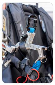
First, attach the webbing carabiner strap through the harness hang point loop or around the side lumbar support strap using a larks foot. Then attach the back up loop (grey) to the back up shackle before passing the main hang point loop (red or blue) through the slot. The carabiner can now be attached through the main hang loop.
