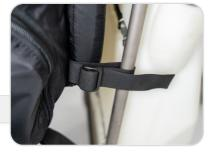
Now attach the mid frame attachment straps to the frame, the paramotor manufacturer should indicate the exact point of connection. Ensure to double lock the buckles.
