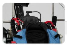
Connect the bridles to the dedicated shoulder attachment points using suitable connectors (not supplied). Ensure the maillons are done up tightly, use pliers but do not over-tighten.
