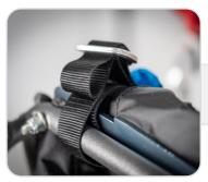
The second method is to pass the metal bar of the paramotor frame through the pre-made loops of the webbing on the upper attachments. It is essential to refer to the paramotor manufacturer's instructions for specific details regarding the preferred method of attachment and any additional recommendations or considerations.
