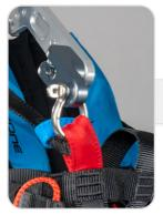
Attach the Indy's main hang points to the paramotor's swing arm or main connection point. This connection point is designed to bear the load and must be connected using a suitable shackle. It is crucial to ensure that the material used is certified for heavy loads.
