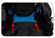
Next attach the lower frame attachment. This webbing needs to pass through the eyelets located inside the harness at the back of the seat plate before attaching to the bottom of the frame (first remove the plastic buckles). The exact point of connection should be indicated by the paramotor frame manufacturer.
