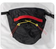
Secure the yellow pins through the yellow loops with the handle correctly positioned as shown. Put the ends of the yellow pins in the flap provided. Ensure the assisting magic string or plastics are removed from the pin loops.
