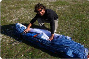
**Step 6.** Fold the wing with 3 or 4 folds whilst being careful not to crush the LE.
