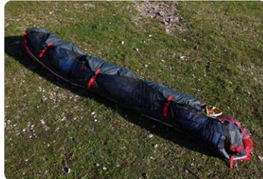
**Step 9.** Turn the Concerto on its side and make the first fold just after the LE reinforcements. Do not fold the plastic reinforcements, use 3 or 4 folds around the LE.
