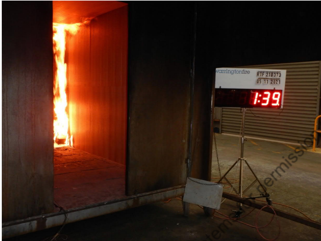
Figure 17 The specimen 1 minute 39 seconds after burner ignition with the burner output of 100 kW
