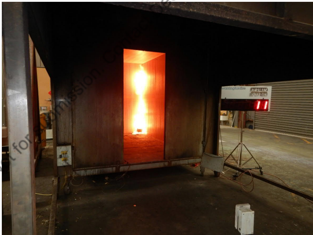
Figure 16 The specimen 11 seconds after burner ignition with the burner output of 100 kW
