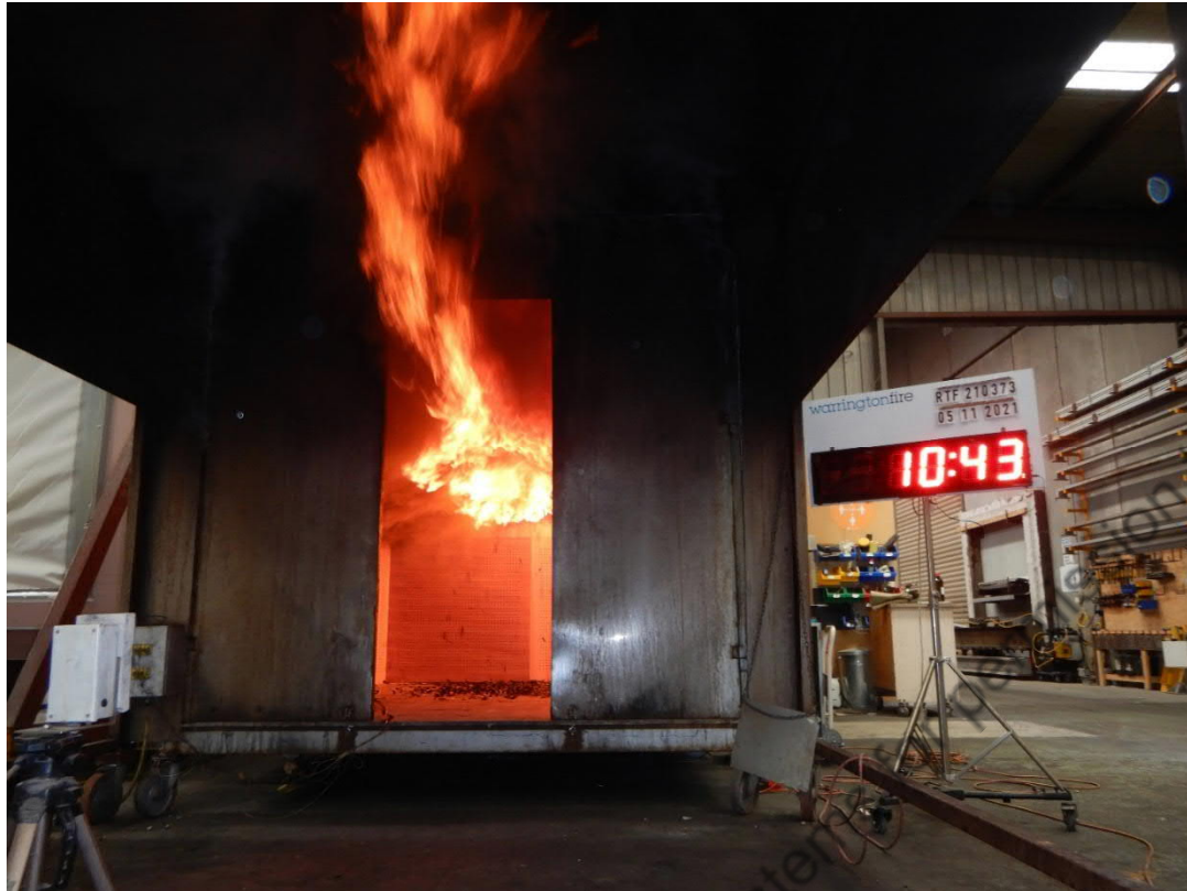
Figure 21 The specimen after flashover (43 seconds after burner output was increased to 300 kW)
