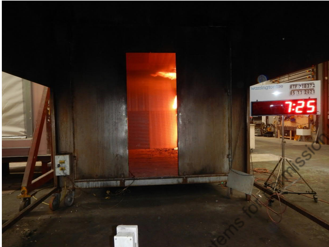
Figure 19 The specimen 7 minutes 25 seconds after burner ignition with the burner output of 100 kW
