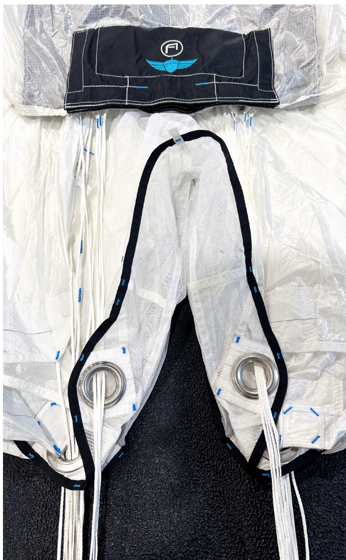
ONLY Control Lines through rear grommets
