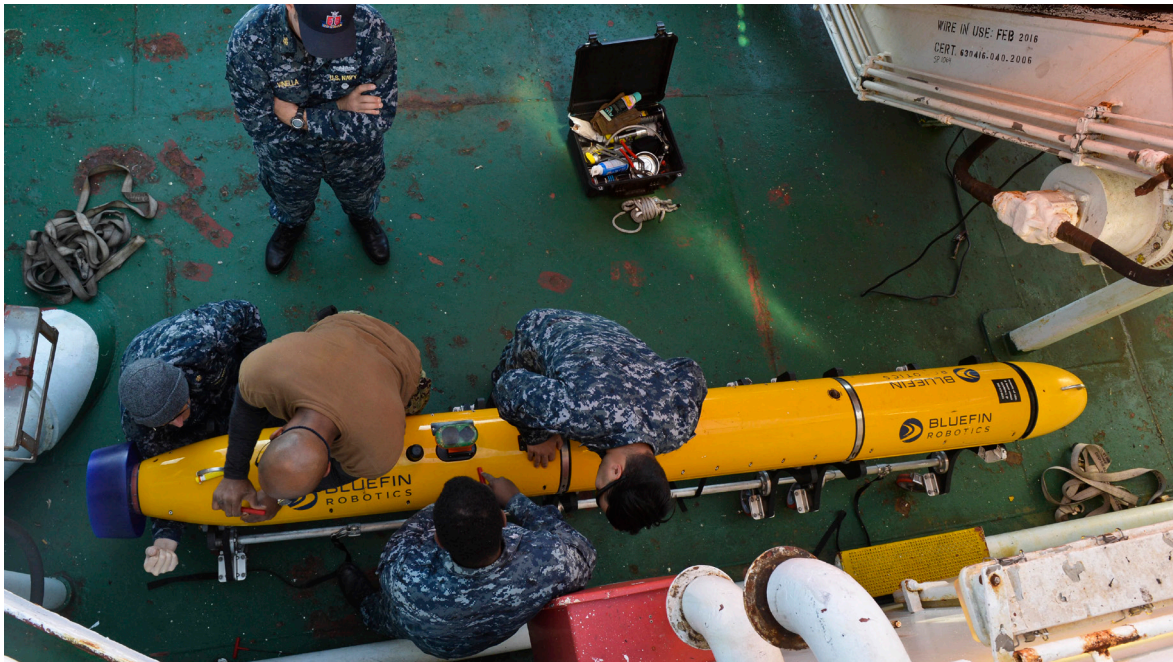
Sailors assigned to Unmanned Undersea Vehicle Squadron 1 (UUVRON 1) perform maintenance on a Bluefin-12D, an unmanned underwater vehicle (Photo: US Navy)
