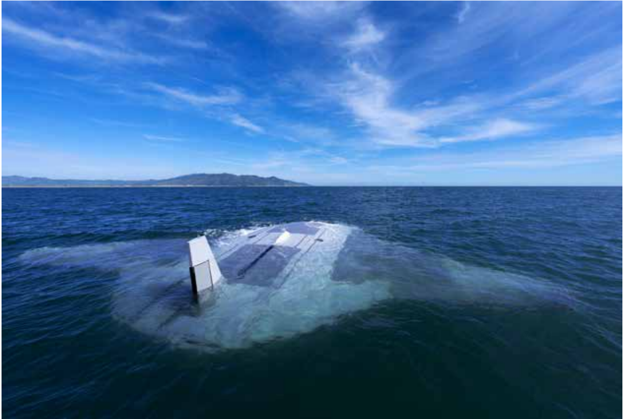
The Extra Large autonomous underwater vehicle 'Manta Ray', developed by the US Defense Advanced Research Projects Agency (DARPA) and Northrop Grumman. Source: Northrop Grumman
