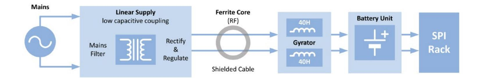
The gyrator circuitry mimics a very large inductor (40 Henry) on every power lead. This prevents interference (like 50 Hz) from getting to the SPI Rack.
