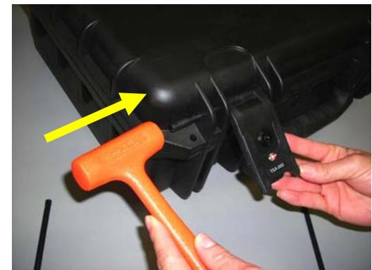
Tap pin back in place to secure latch. Actuate latch to make sure it operates smoothly
