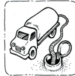
Vacuum truck emptying a septic tank (Credit: AKVO, nd)
