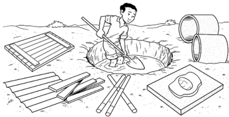
Digging a pit may not be possible if the groundwater level is very high
