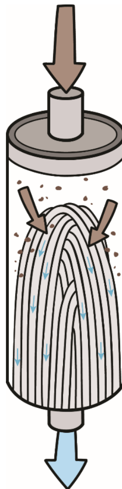
Figure 5. Example of a hollow fibre membrane. Untreated water (brown arrows) moves into the cartridge and travels through tiny pores in the walls of the hollow fibres. Treated water (blue arrows) then flows through the hollow fibres and out of the cartridge.
