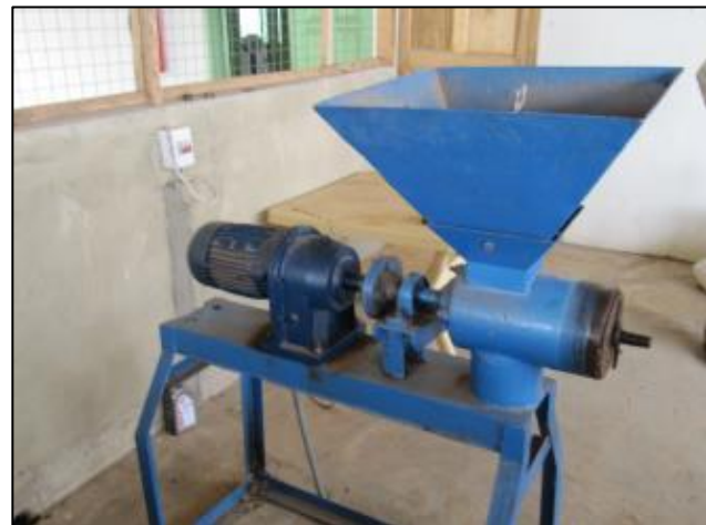
Pelletizers in Uganda and Ghana (Credit: Eawag-Sandec)
