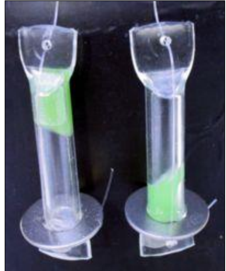
Water Pasteurization Indicator (WAPI) (Credit: Solar Cooker International)
